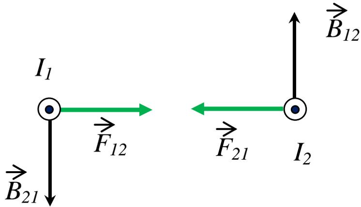
$$F_{12} = I_1 B_{21} L \quad B_{21} = \frac{\mu\mu_0}{2\pi} \frac{I_2}{R} \quad F_{12} = \frac{\mu\mu_0}{2\pi} \frac{I_1 I_2}{R} L$$
